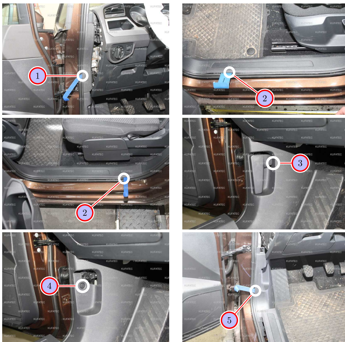
Figure 9: Removing trim panel driver's side
